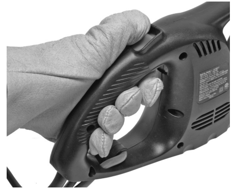
Figure 3-7: Squeezing trigger switch to start trimmer
